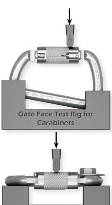
Side Load Test Rig for
